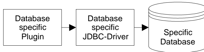
Figure 9-1 JDBC Driver Layers
